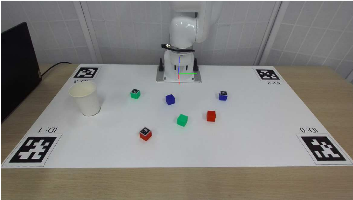
Figure 4: Visualization of the estimated robot base frame origin.
